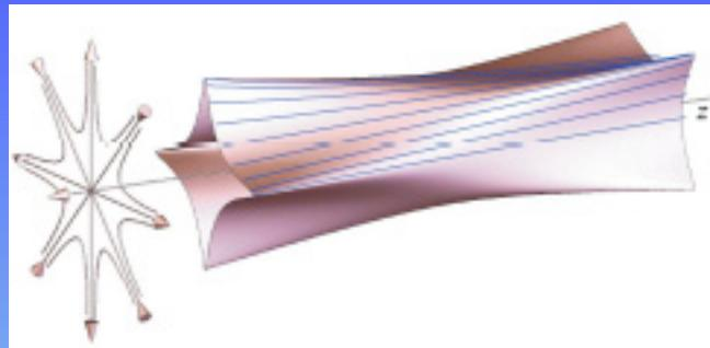
FIG. 2: Magnetic field from the octupole and solenoid coils. The vectors on the left represent the directions of the axially-invariant field from these coils. The surface is created by following the field lines from a radially centered circular locus; the lines shown within the surface are field lines.
