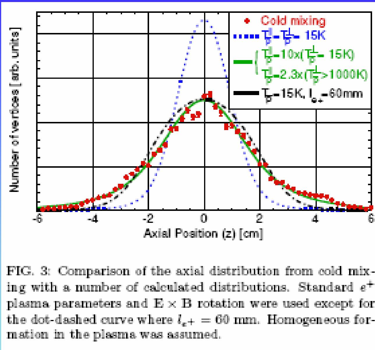
FIG. 3: Comparison of the axial distribution from cold mixing with a number of calculated distributions. Standard  $e^+$  plasma parameters and  $E \times B$  rotation were used except for the dot-dashed curve where  $l_{e+} = 60$  mm. Homogeneous formation in the plasma was assumed.
