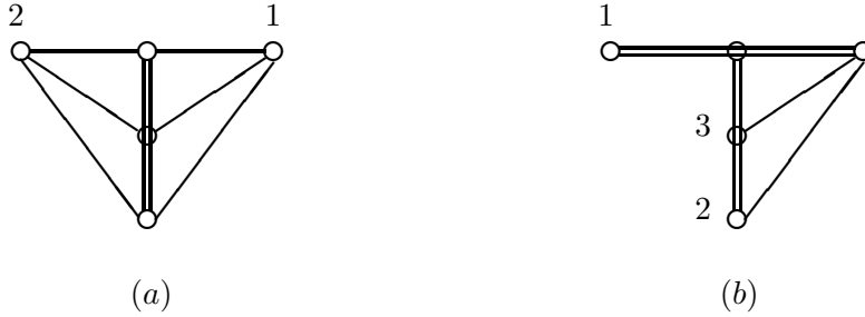
Figure 3: Two non-generic frameworks with 5 vertices in \mathbb{R}^2 . Framework (a) is not globally rigid even though it has only one missing edge, namely (1,2). On the other hand, framework (b) is universally rigid even though it has two adjacent missing edge, namely (1,2) and (1,3).
