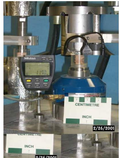
Figure 3. The uniaxial test frame, showing load cell, strain gauge and sample holder
