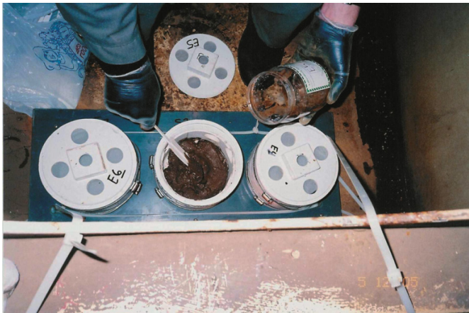
Fig. 1. Sediment is placed into polyvinyl chloride (PVC) incubation chambers moored to the bottom of a ballast tank.
