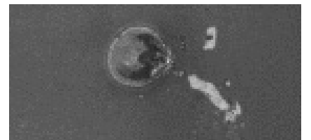
(Right) Burned adhesion zone around resistance weld. Exhaust vapor channel is clearly visible.
