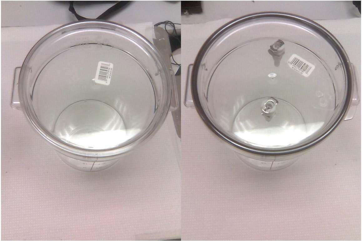
Figure 2.2 Illustration of microcosm container design with unmodified (left) cover for oxic conditions, and modified (right) cover for simulated anoxic conditions.
