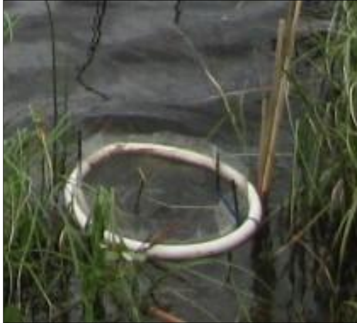
Figure 2.1: Photo of floating hoop emergence traps (Photo by K. Jurkowski, 2009) Hoop diameter is 30 cm.
