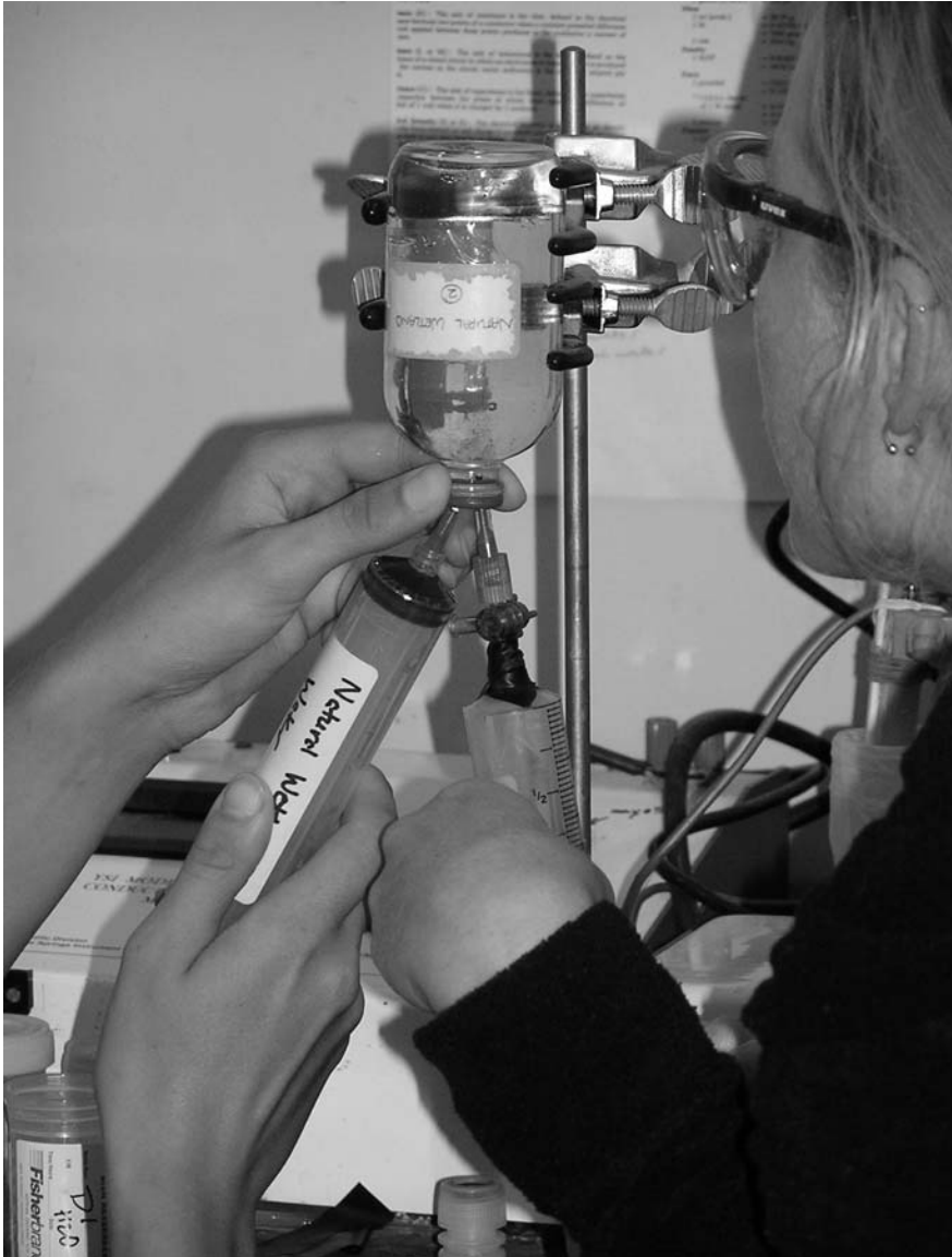
Figure 2.3 – Withdrawing a portion of wetland water and replacing with ultrapure helium using gas-tight syringes.
